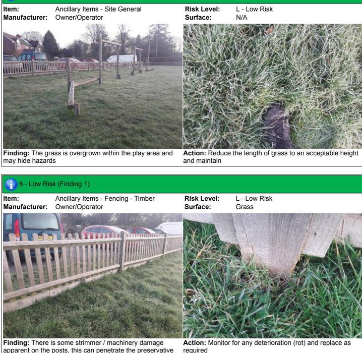
apparent on the posts, this can penetrate the preservative applied to the timber and accelerate the rotting process
