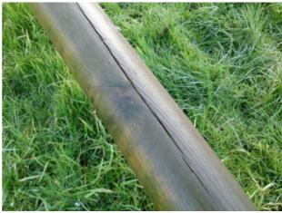
Finding: The timber has a number of air cracks
