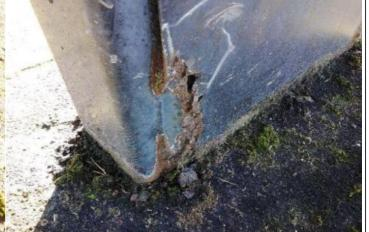
**Finding:** Parts of the steel on this item have corroded excessively and the metal has perforated in places
